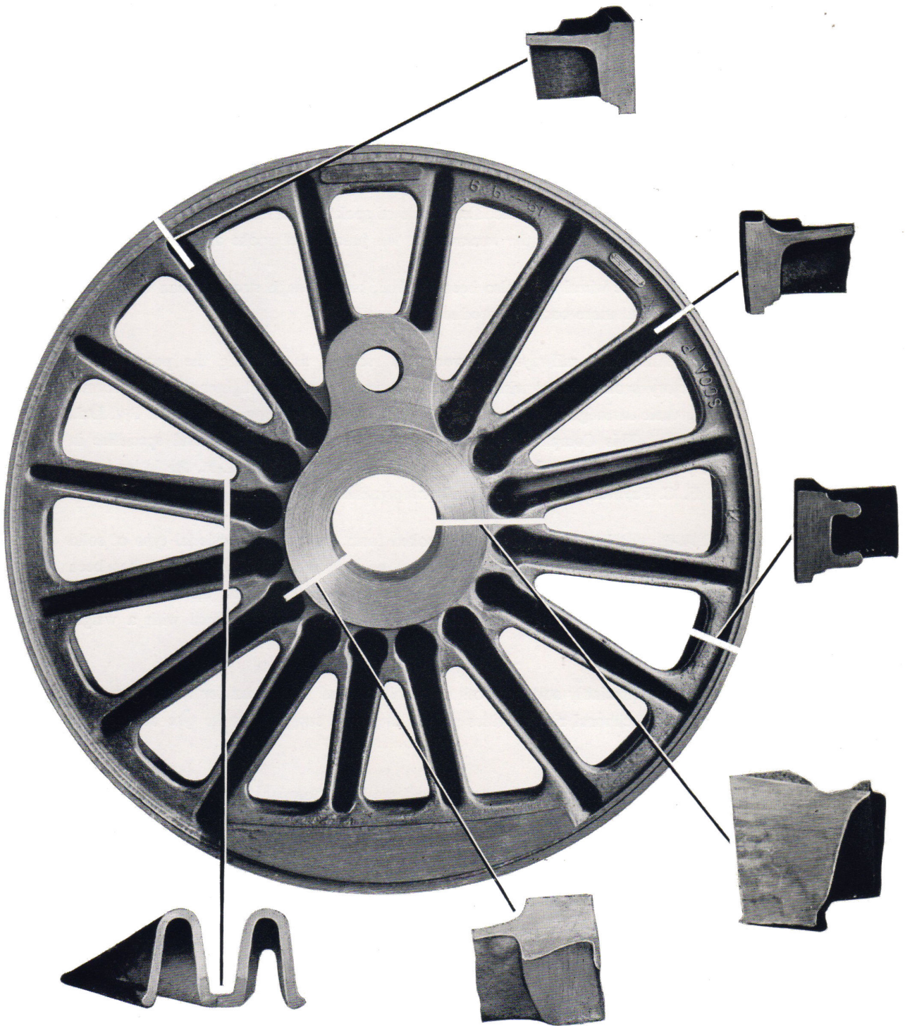
View of typical S.C.O.A.-P. wheel centre showing various sections
