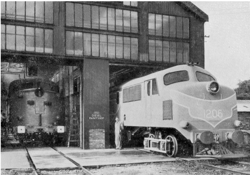
1,500 h.p. Diesel Electric Locomotive on accommodation bogies leaving Spray Booth
