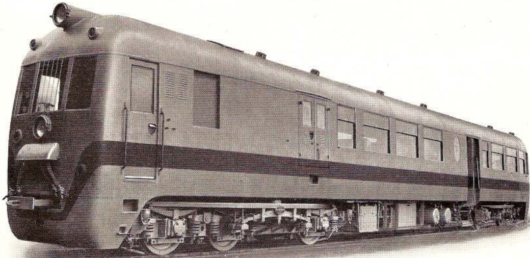
250-275 B.H.P. Diesel Mechanical Rail Coach, New Zealand Government Railways.
