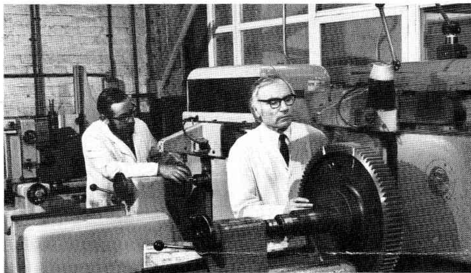
Peter Grainger, nearest the camera, and Alan Smith flank profile checking.
